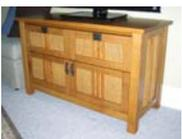
**A/V Cabinet.** Made of quarter sawn White Oak with mission finish, holds all A/V components including center channel and base speakers, doors have rattan centers instead of panels to allow for ventilation and sound transfer, mortise and tenon construction (74 mortise and tenon joints counting cabinet frame and doors), upper sliding shelves and “secret” side doors with automatic interior lights for accessing back of components.
